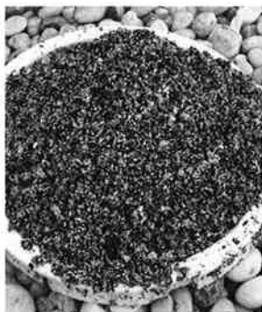
Deviating from a free draining system, small bins were buried in the roof to test the characteristics of a green roof that retains storm water to the full capacity of the soil.
