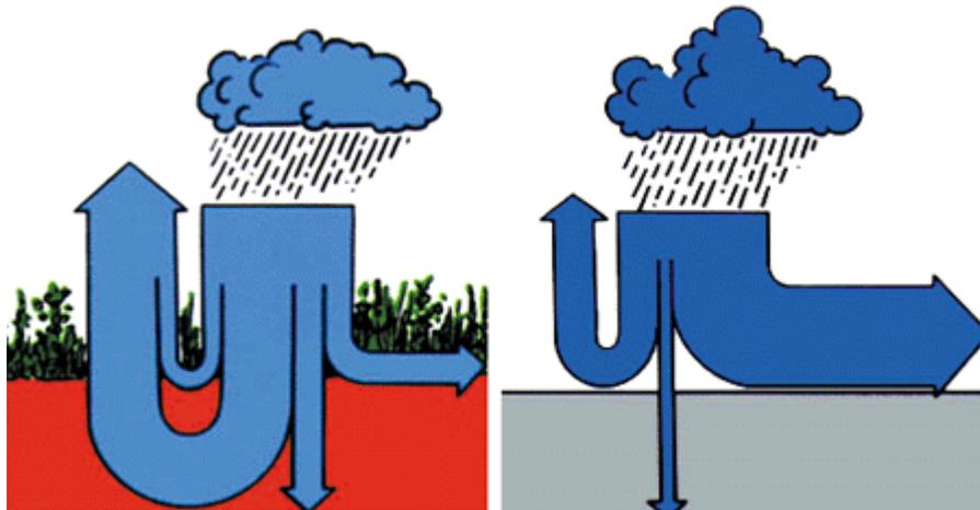
*Figure 1: When rain falls on forested and open, undisturbed land, about 30% reaches shallow aquifers, another 30% nourishes deeper aquifers, and approximately 40% is returned into the atmosphere. There is rarely any surface runoff. In metropolitan areas, a staggering 75% of the rainwater becomes surface runoff. Illustration courtesy of Bauverlag GmbH, Germany.\**
