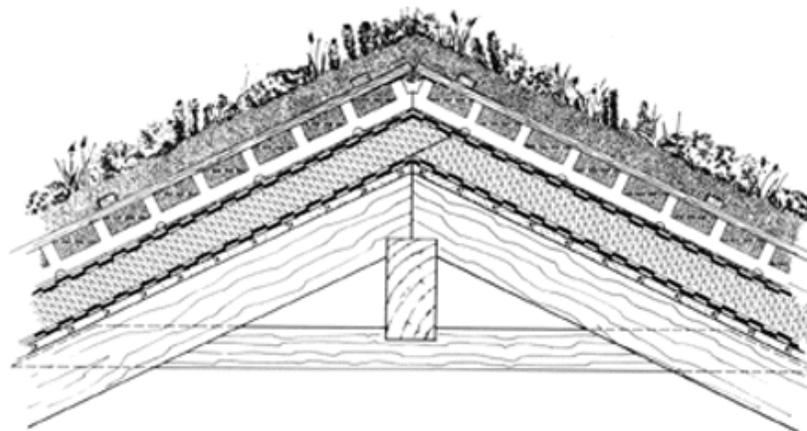
*Figure 2. A roof slope between five and 20 degrees is ideal for a green roof because it allows the water to drain naturally. Illustration courtesy of Bauverlag GmbH, Germany.\**
